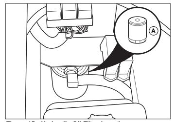
Figure 15. Hydraulic Oil Filter Location
